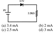
10. The diode used in the circuit shown in the figure has a constant voltage drop of 0.5 V at all currents and a maximum power rating of 100 milliwatts. What should be the value of the resistor R, connected in series with the diode for obtaining maximum current -
