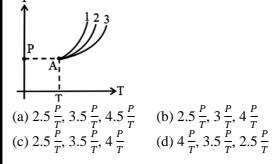
47. Heat is supplied to a diatomic gas at constant pressure. The ratio of  $\Delta Q : \Delta U : \Delta W$  is -
