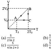
16. An ideal gas is taken through the cycle  $A \rightarrow B \rightarrow C \rightarrow A$ , as shown in the figure. If the net heat supplied to the gas in the cycle is 5 J, the work done by the gas in the process  $C \rightarrow A$  is-
